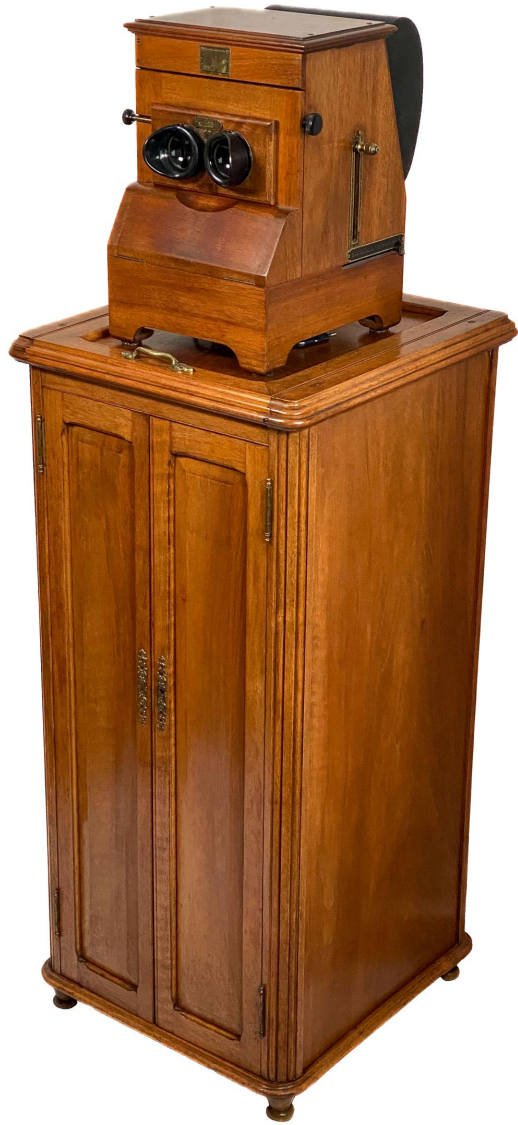
Planox Stéréoscope Magnétique on a storage cabinet. The stereoscope has a illumination device attached.
