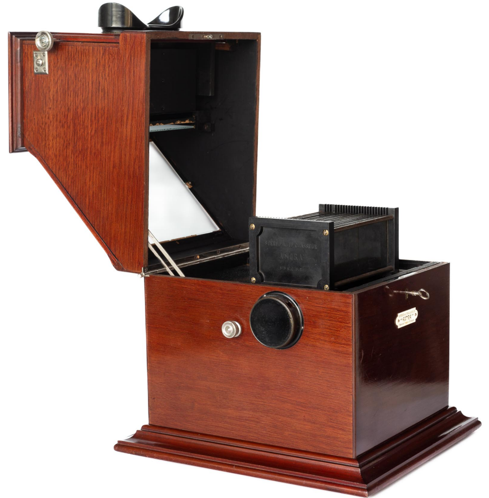
An opened Astra 6 x 13 stereoscope with the slide tray visible. Pulling out the small silver knob activates the autochrome-mode.
