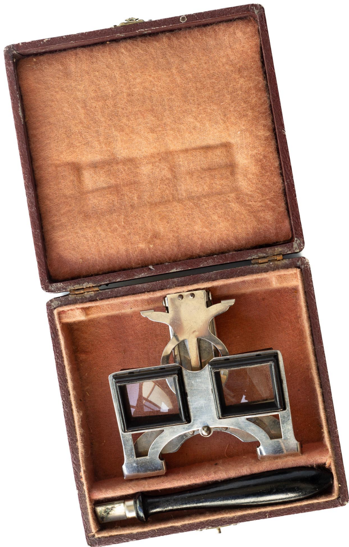
L'Omnium with rectangular prism lenses, stored in its case.
